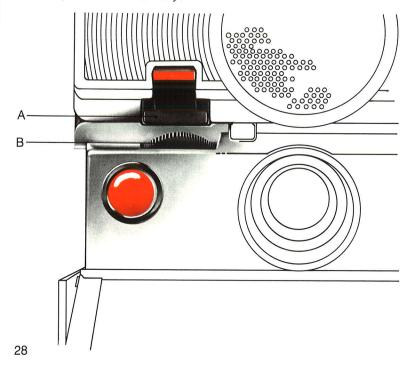
To use the focus wheel: Look at the most important part of the scene. Roll the focus wheel all the way in one direction, then all the way in the other. Notice that the image changes from fuzzy to sharp and back to fuzzy.
